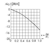
Fig. 4 · Diagram of valve-specific correction terms
