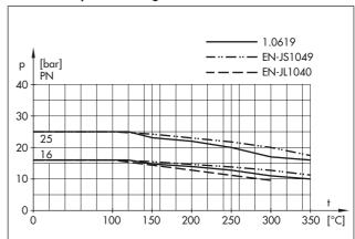
The permissible pressures, differential pressures and temperatures are restricted by the specifications in the pressure-temperature diagram.
